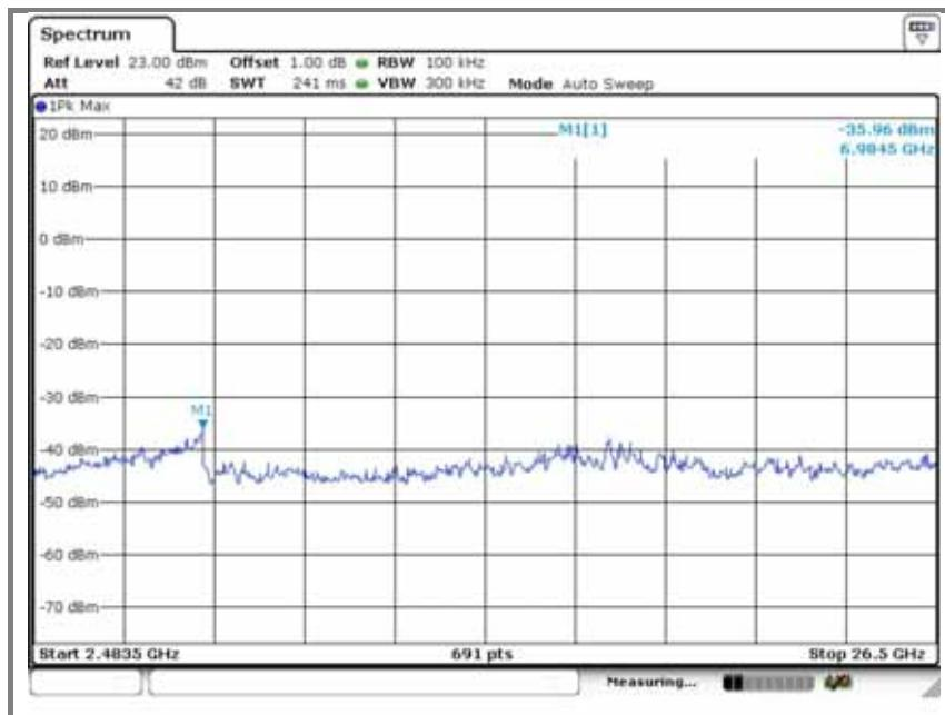
**Operation mode: BLE mode (Port2)****A. Low channel****Reference level measurement**
