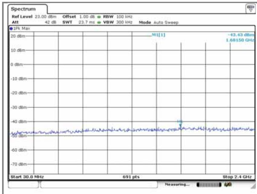
**Emission level measurement 2**
