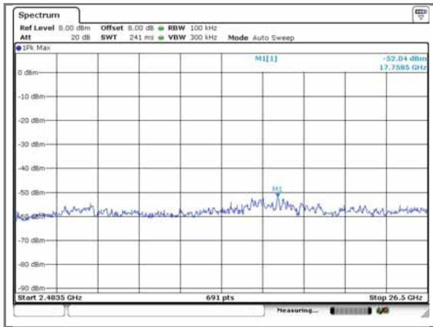
**C. High channel****Reference level measurement**
