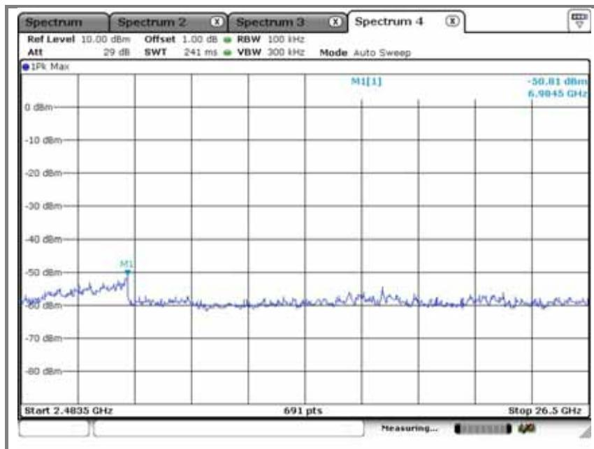
**Operation mode: 802.11b mode (Ant 2)****A. Low channel****Reference level measurement**
