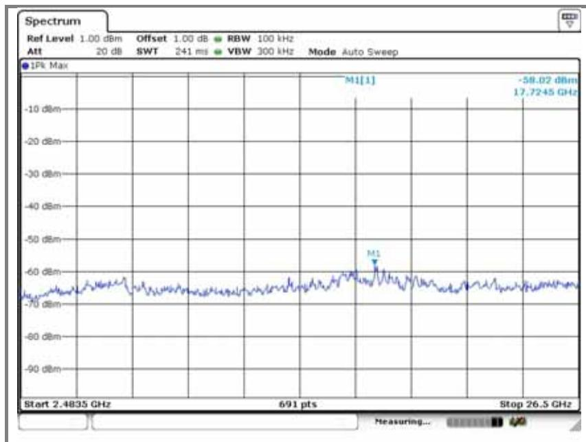
**Operation mode: 802.11g mode (Ant 1)****A. Low channel****Reference level measurement**
