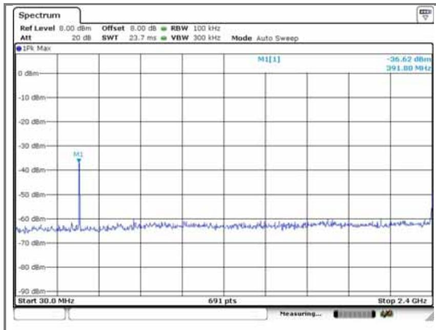
**Emission level measurement 2**
