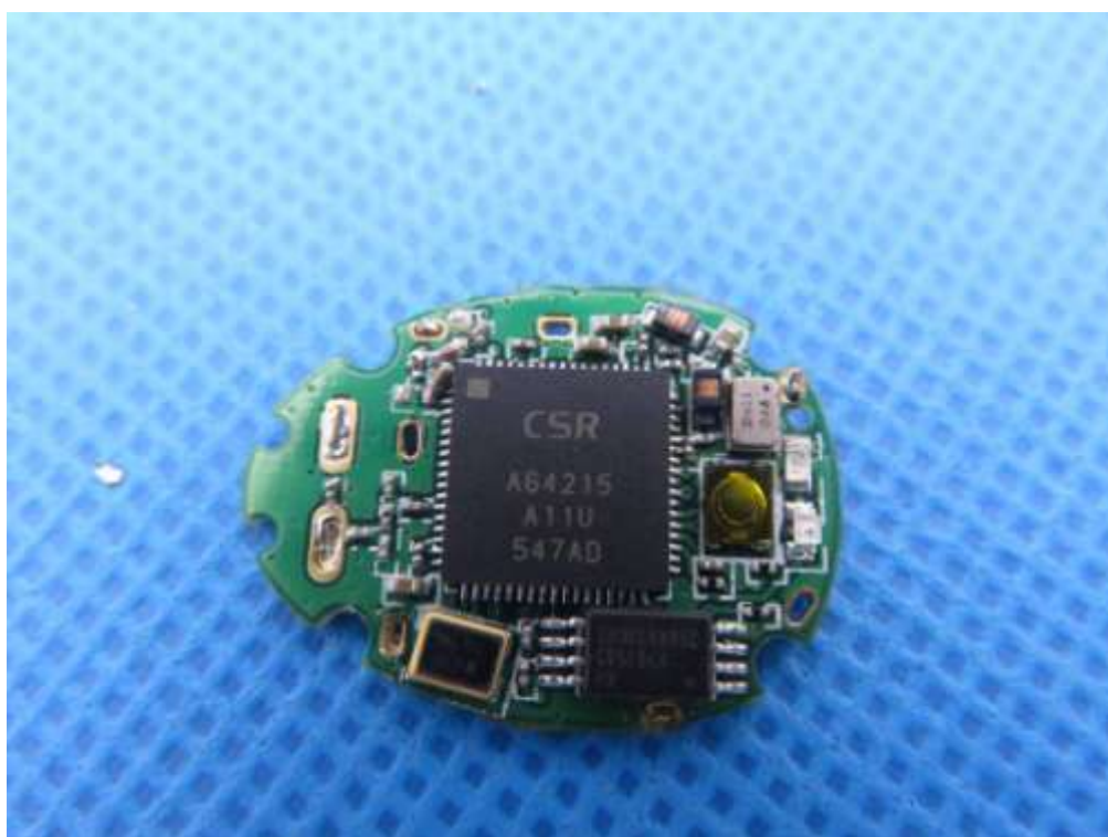
INTERNAL VIEW OF EUT-3 (Second Earbud)
