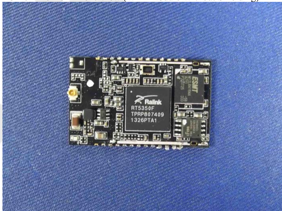
Figure 13 PCB of The EUT-Front View (WiFi Module Without Shielding)
