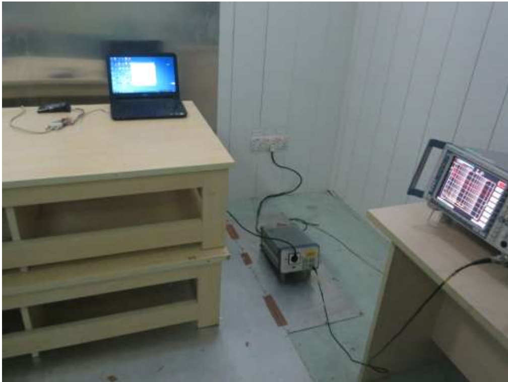
FCC RADIATED EMISSION TEST SETUP
