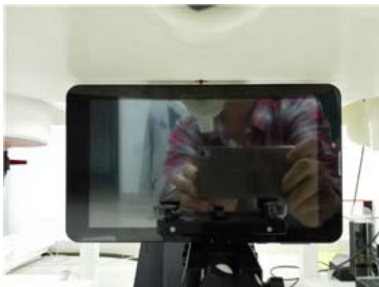
0mm Body-worn Left Side Setup Photo
