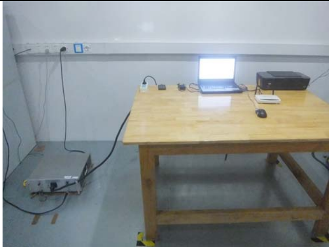
Conducted Emissions Test Setup – Front View
