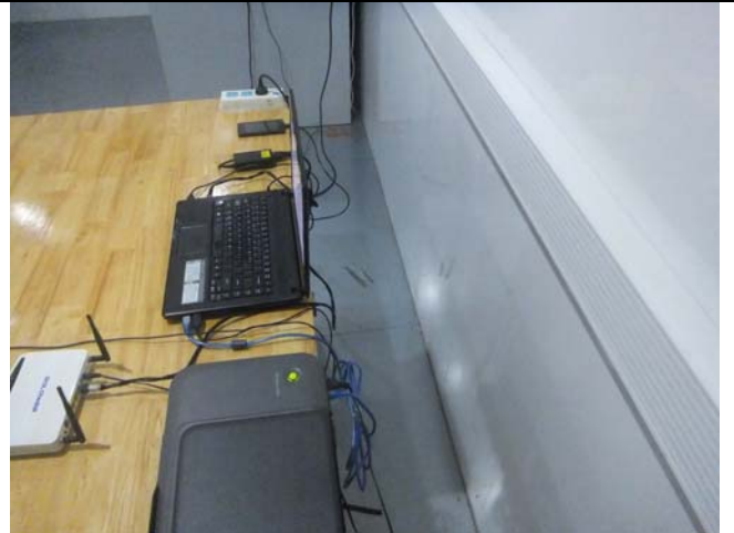
Conducted Emissions Test Setup – Side View
