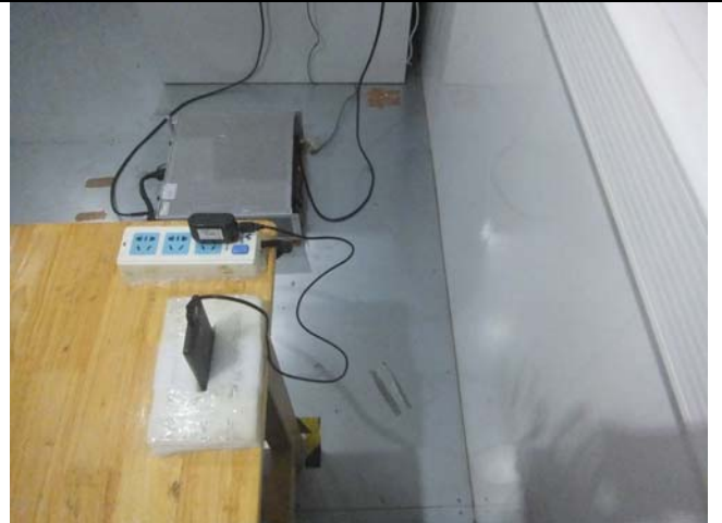
Conducted Emissions Test Setup Side View
