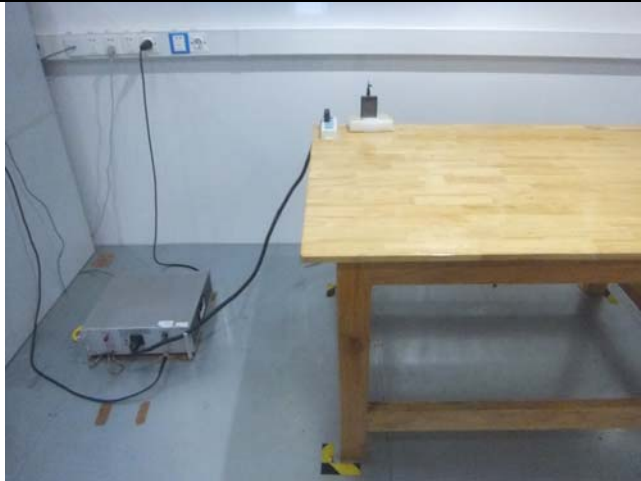
Conducted Emissions Test Setup Front View
