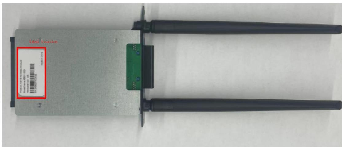
The label is attached to the surface of the shield with a permanent adhesive.
