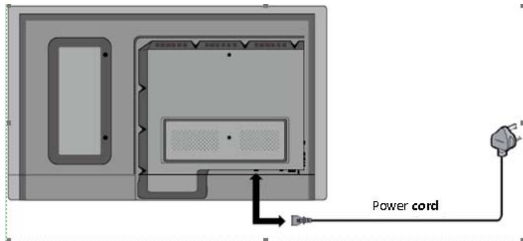
**Step 2** Connect the panel to the power supply. Switch on the rocker switch (on the right bottom of the rear of the panel, next to the power port) to enter the standby status. The power indicator turns red.
