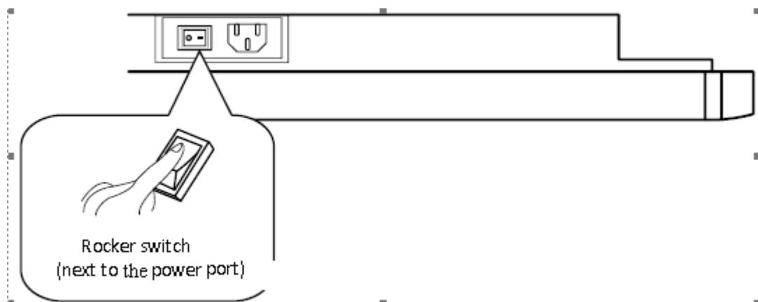
**Step 3** Press power switch on the control panel or **Power** on the remote controller to turn on the interactive panel. The OPS is started. The power indicator turns green.
