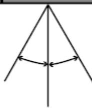
The effective receiving distance is about 5 meters from the front of device.
