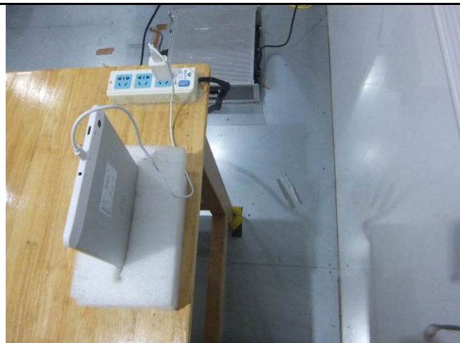
Conducted Emissions Test Setup Side View
