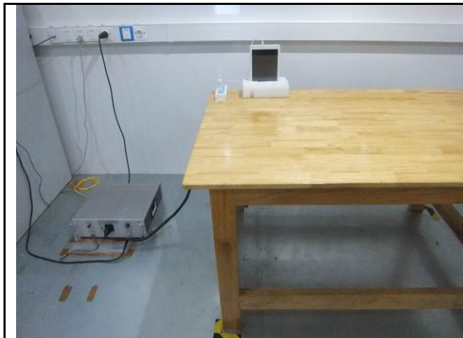
Conducted Emissions Test Setup Front View
