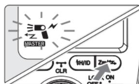
Short press the [MODE] button on the master control unit, the flash mode will switch among ETTL, M, and Multi.
