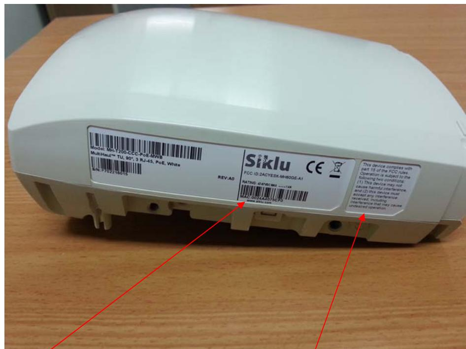
Label with FCC ID:2ACYESK-MH60GE-A1 location, label with the statement according to FCC part 15 §15.19(a)(3)
