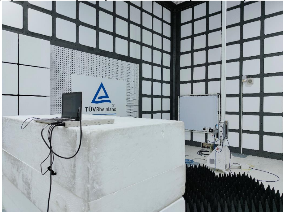
Photograph 6: Test Setup for Spurious Emissions (Back View 4)
