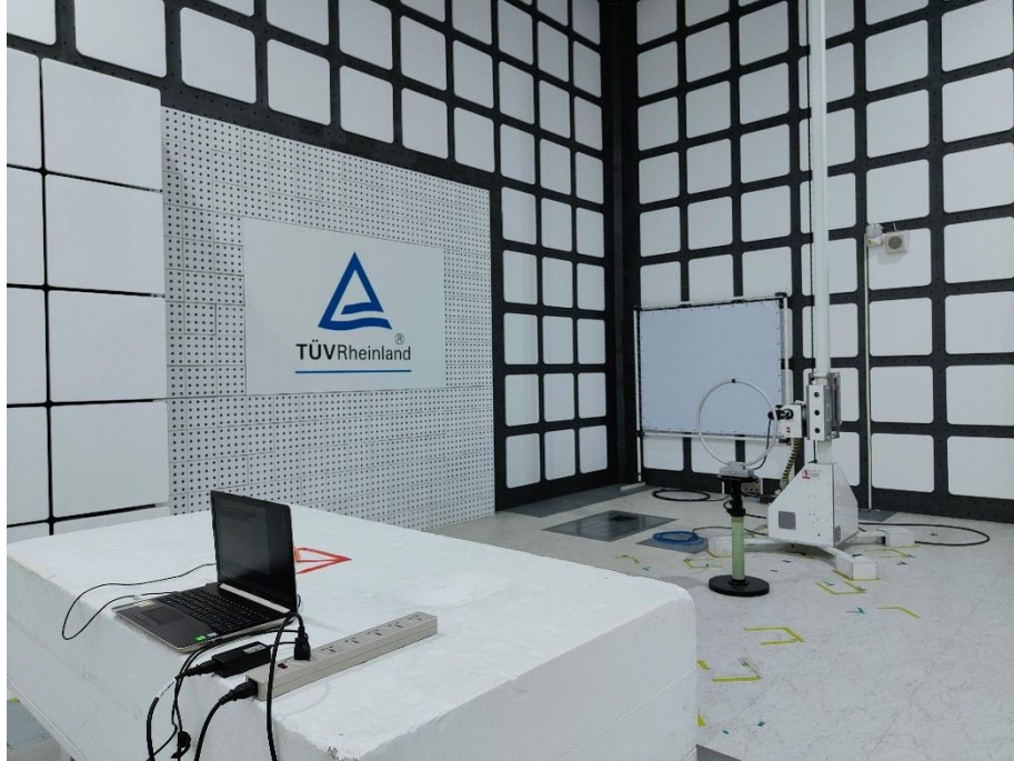
Photograph 3: Test Setup for Spurious Emissions (Back View 1)
