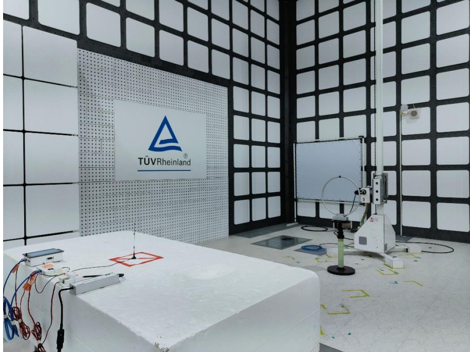
Photograph 9: Test Setup for Spurious Emissions (Back View 1)
