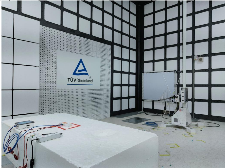
Photograph 4: Test Setup for Spurious Emissions (Back View 2)
