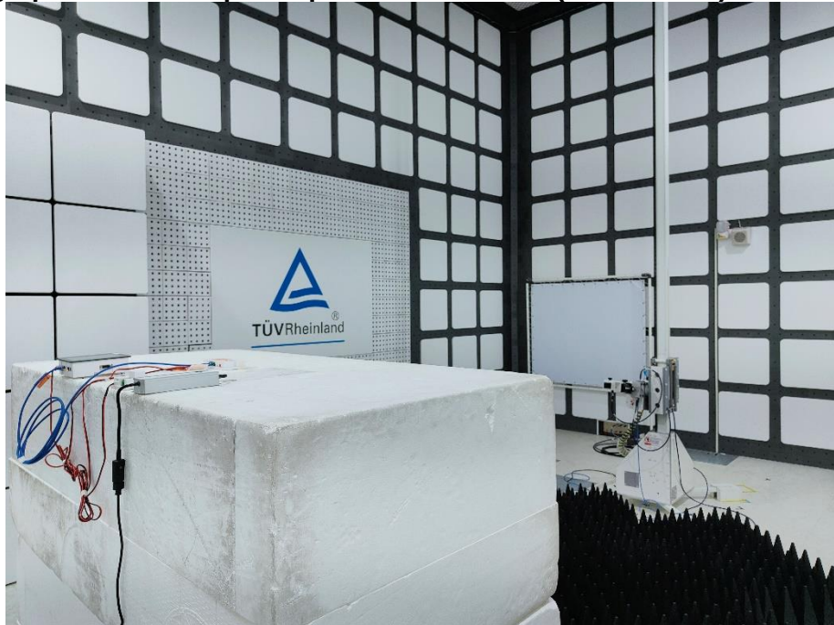
Photograph 6: Test Setup for Spurious Emissions (Back View 4)
