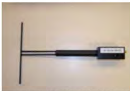
Figure 1 – Satimo COMOSAR Validation Dipole
