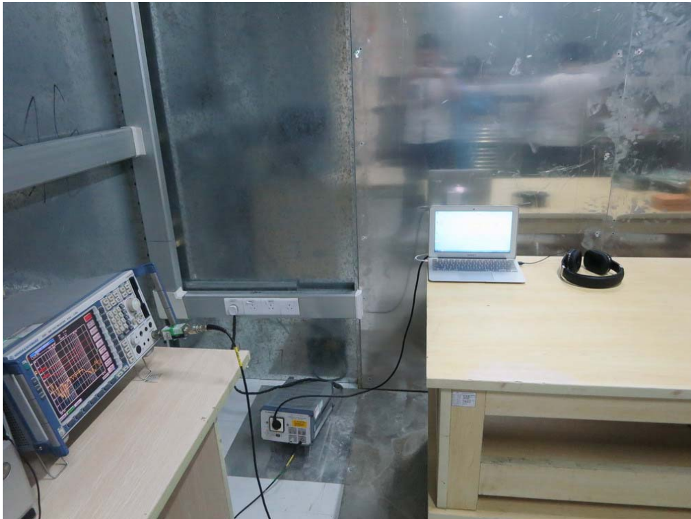
FCC RADIATED EMISSION TEST SETUP
