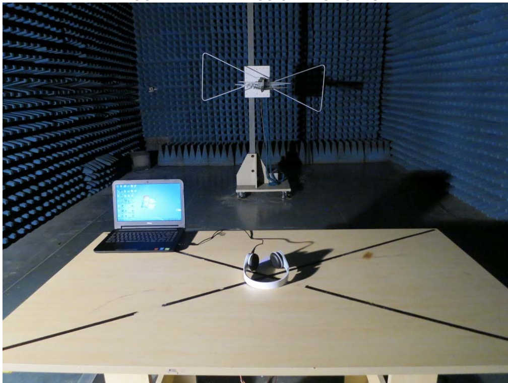
FCC RADIATED EMISSION TEST SETUP
