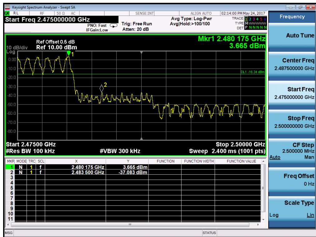
EDR mode ( $\pi/4$ -DQPSK): Band Edge-Left Side
