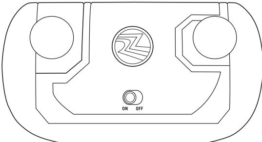
Use the ON/OFF switch to turn your CONTROLLER ON. The center logo will be flashing first each time the power is turned on. Then the logo light will turn steadily on when pairing is successful.
