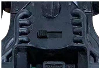
Use the switch on the bottom of your CHASSIS to turn on the CHASSIS and pair with your CONTROLLER.
