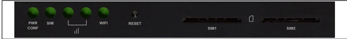
Figure 5: LEDs on the GW1000M Series router
