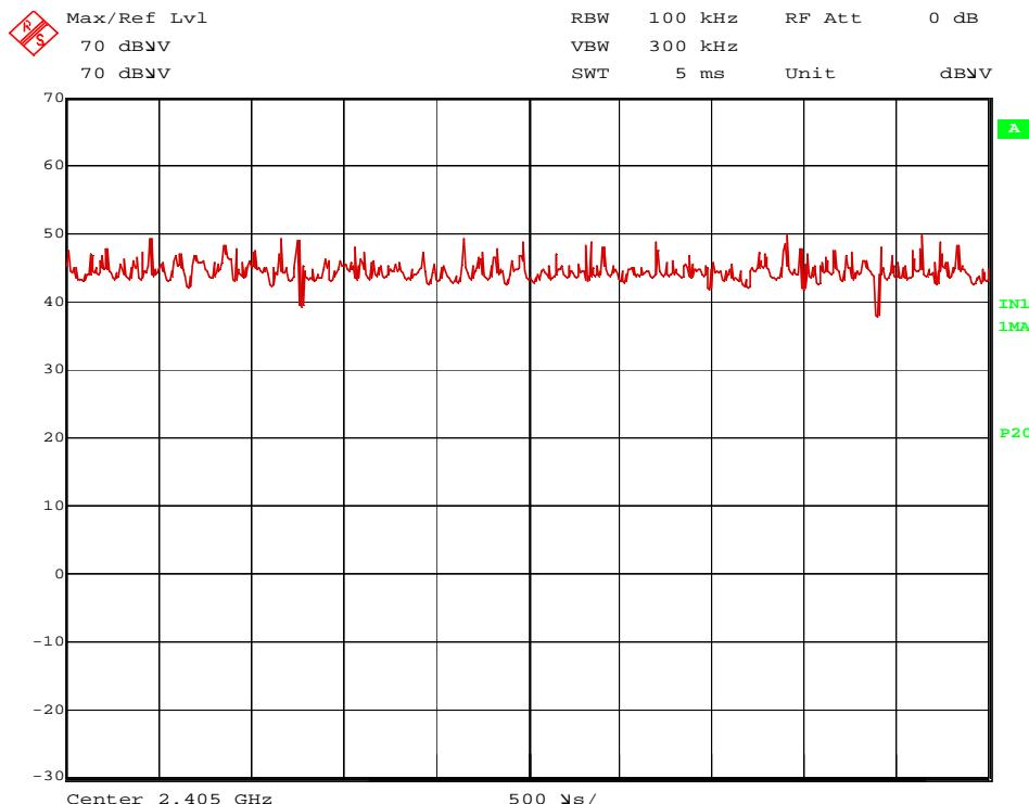
The EUT is transmitting data continuously in test mode. Therefore no duty cycle correction or similar measurement techniques have to be used.
