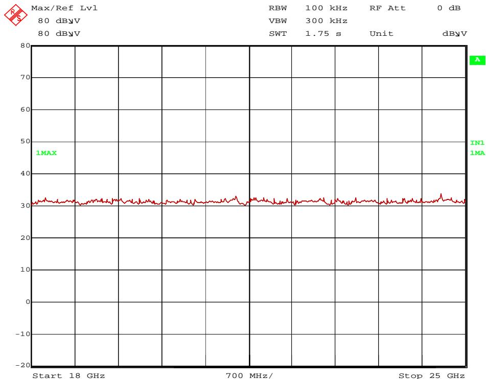
145863\_SpurEmiss\_Pos1\_Ver\_ch26\_18-25GHz.wmf: Spurious emissions from 18 – 25 GHz
