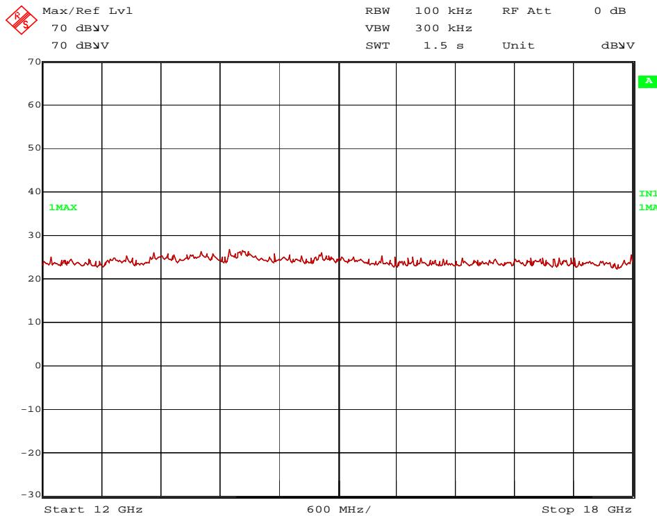
145863\_SpurEmiss\_Pos1\_Hor\_ch26\_12-18GHz.wmf: Spurious emissions from 12 to 18 GHz
