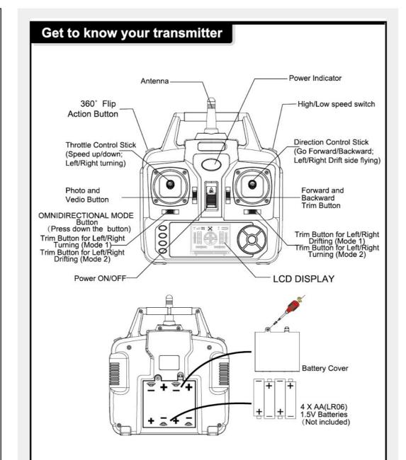
LCD DISPLAY TOTAL MODE I ES 1.Drift Left/Right Flying Trim (Mode 1) / Turn Left/Right (Mode 2) 03.Turn Left/Right Trim (Mode 1) / Drift Left/Right Flying Trim (Mode 2) 04.Throttle Speed 05/06/07/08. Direction Control Display 09/10.Turn Direction 1.High/Low speed 2.Battery Strength for Transmitter 3.MODE 14. Singal strength between quadcopter and transmitter. INSTALL LANDING SKIDS & GUARDS
