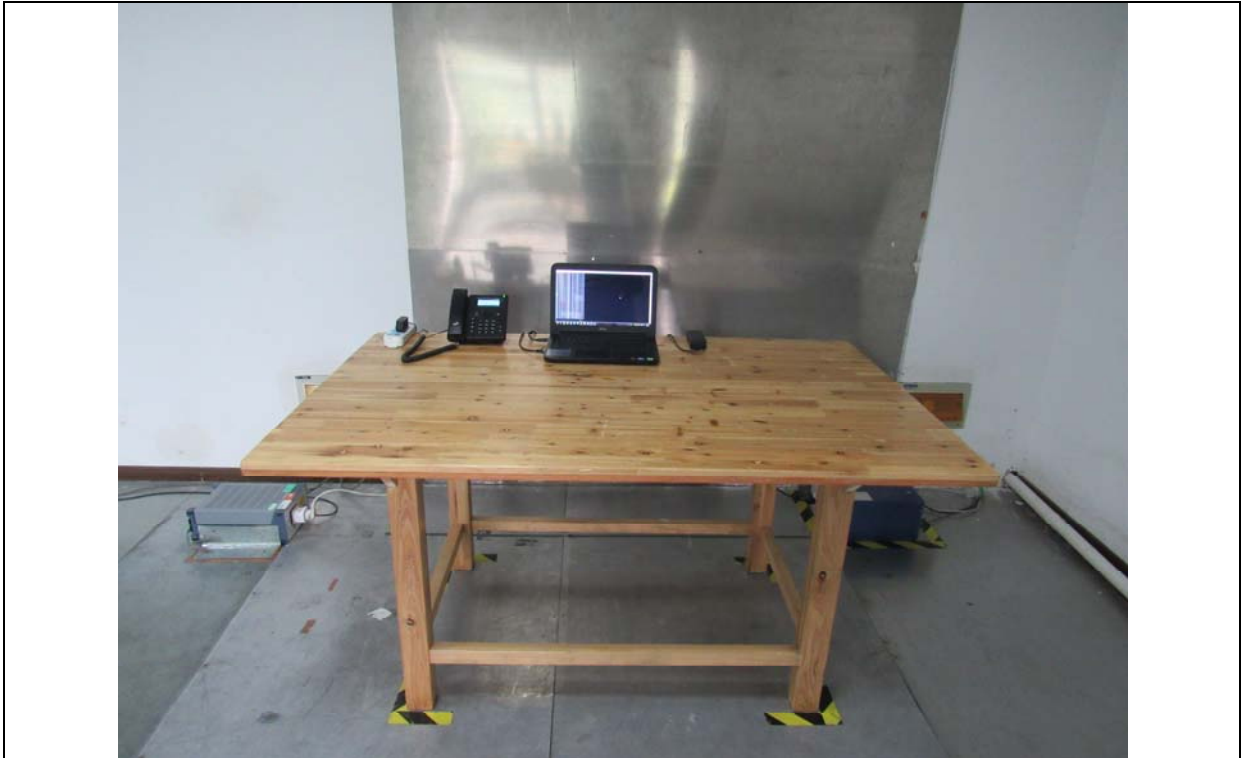
Conducted Emissions Setup Front View
