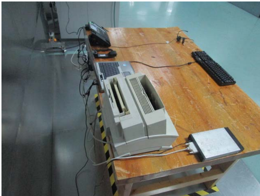
Conducted Emissions – Side View (Charging from POE)
