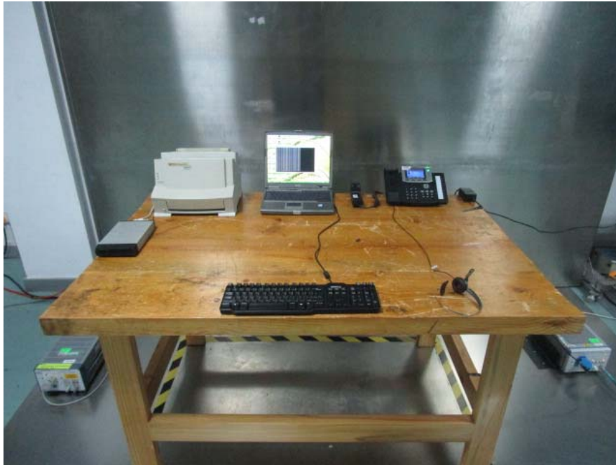
Conducted Emissions - Front View (Charging from POE)
