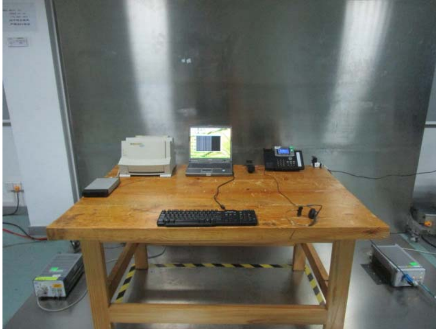
Conducted Emissions - Front View (Charging from Adapter)
