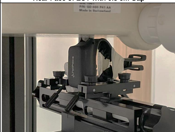
Right Side of EUT with 0.5 cm Gap
