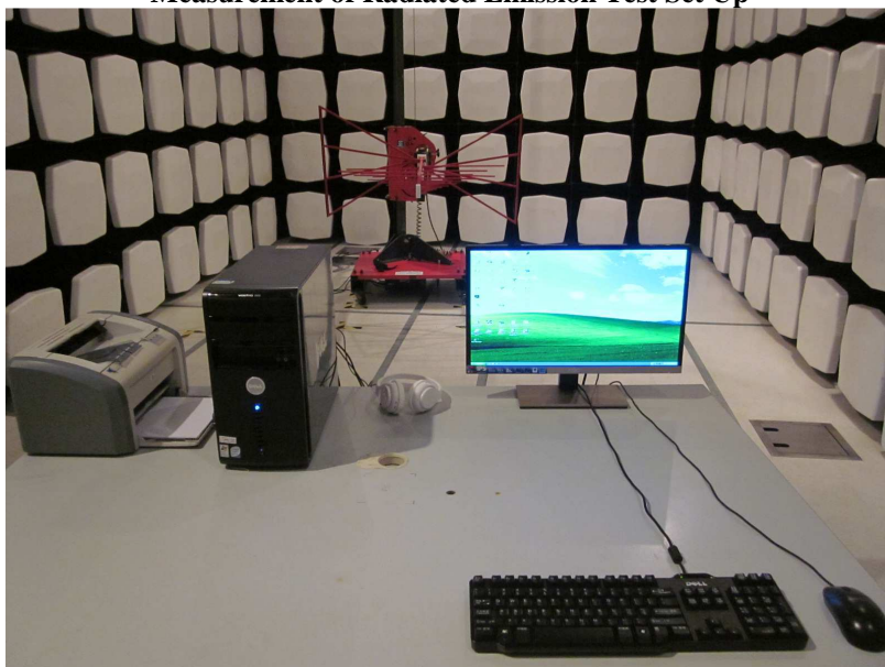
Measurement of Radiated Emission Test Set Up
