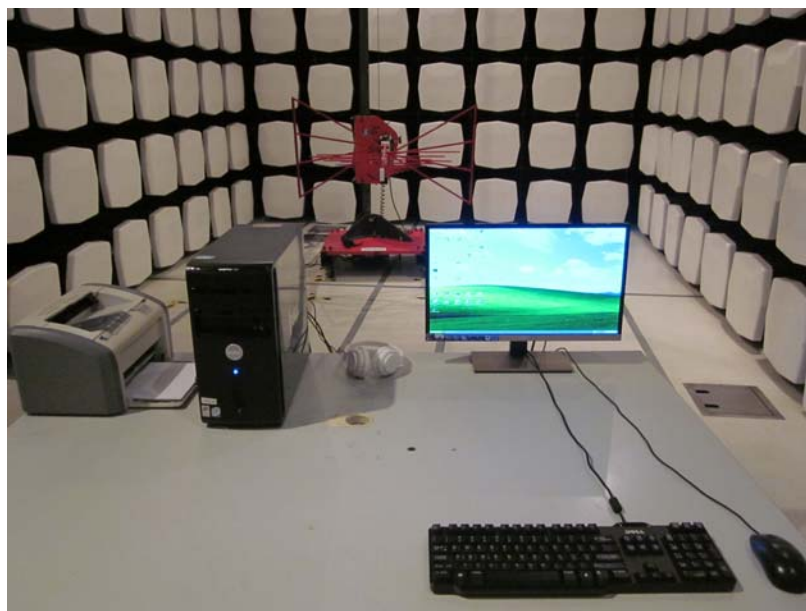
Measurement of Radiated Emission Test Set Up
