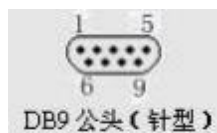
Figure 4. RS232 Pin Definition(Male/Needle Type)
