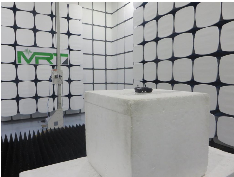
Description: Radiated Emission Test Setup (18GHz ~ 25GHz)
