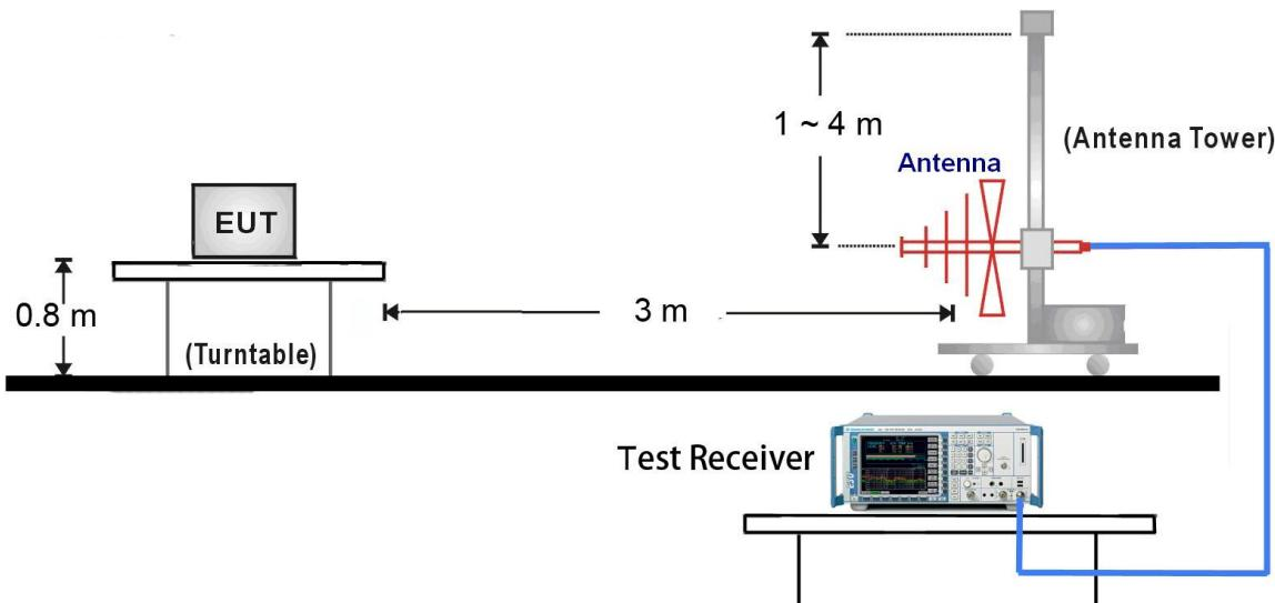
1GHz ~ 25GHz Test Setup:
