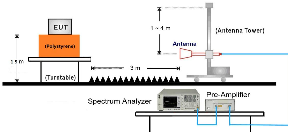
18GHz ~25GHz Test Setup:
