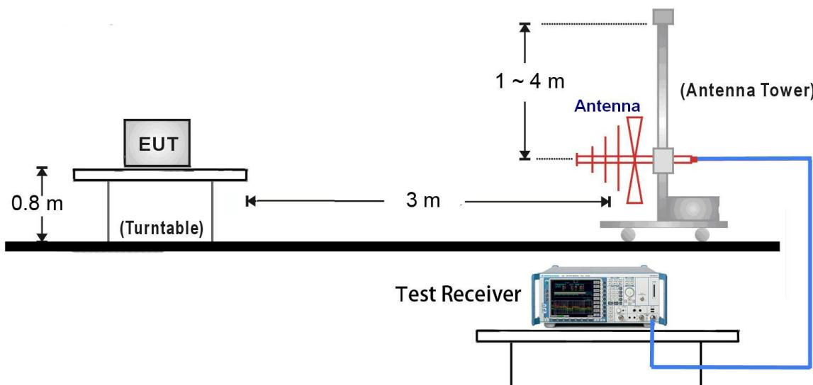
1GHz ~ 18GHz Test Setup:
