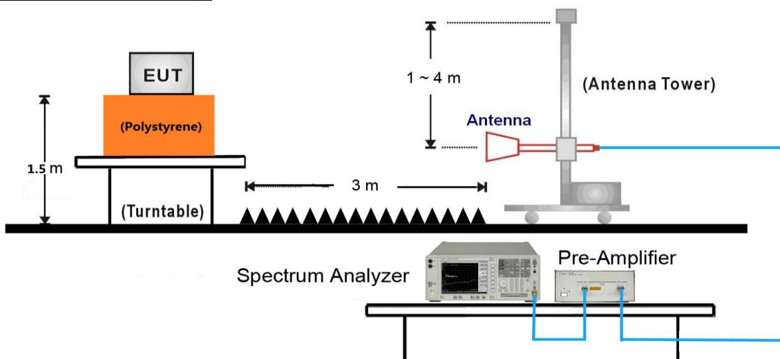
18GHz ~25GHz Test Setup:
