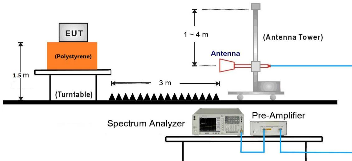
18GHz ~25GHz Test Setup:
