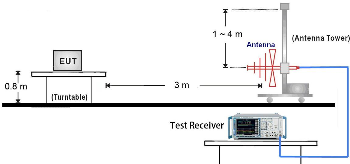
1GHz ~ 18GHz Test Setup:
