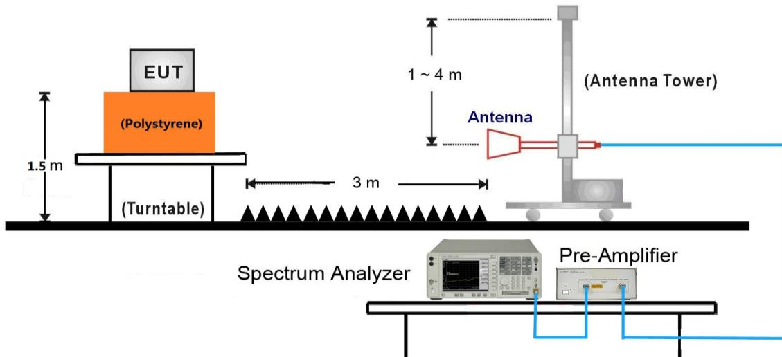
18GHz ~25GHz Test Setup:
