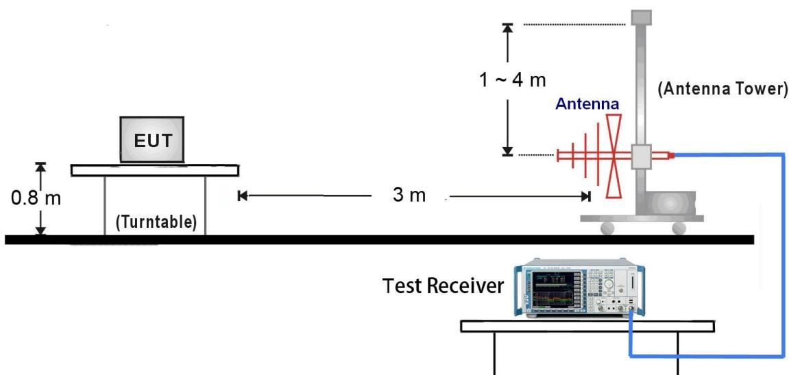
1GHz ~ 18GHz Test Setup:
