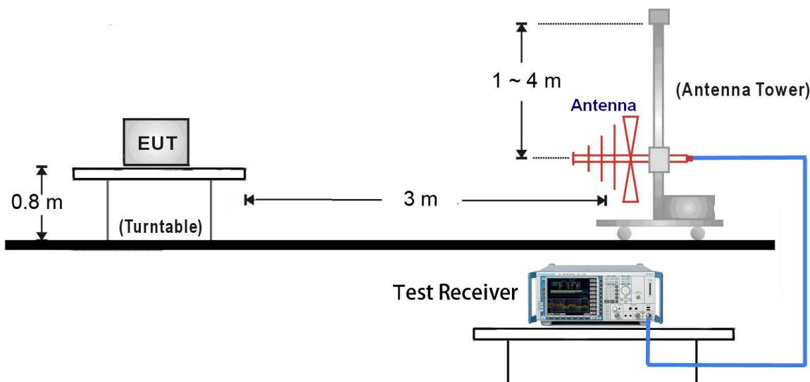
1GHz ~ 18GHz Test Setup:
