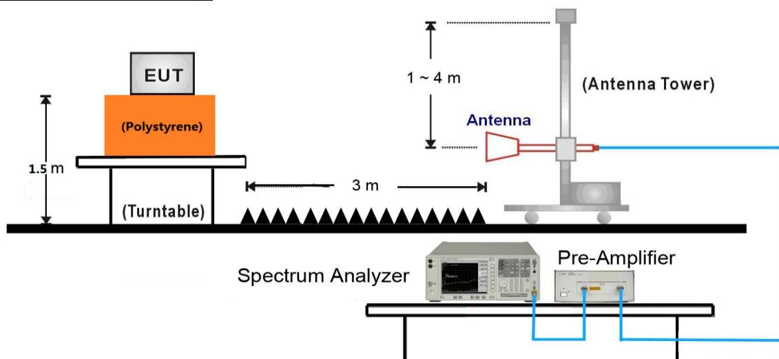
18GHz ~25GHz Test Setup:
