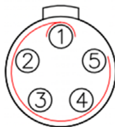
Figure 7 HJ394 C Port Welding Surface View
