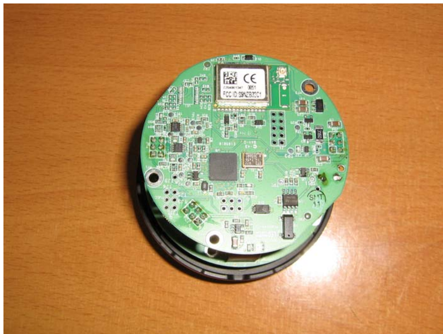
ASM0115 Module installed onto LED Roadway PCB
