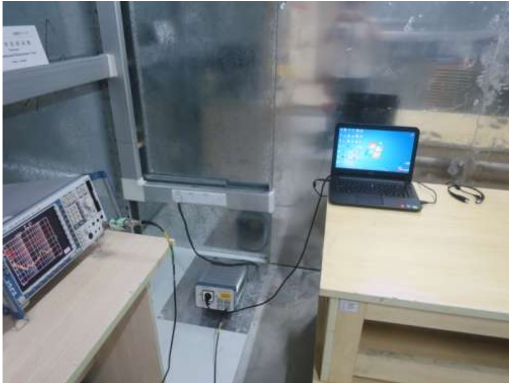
FCC RADIATED EMISSION TEST SETUP
