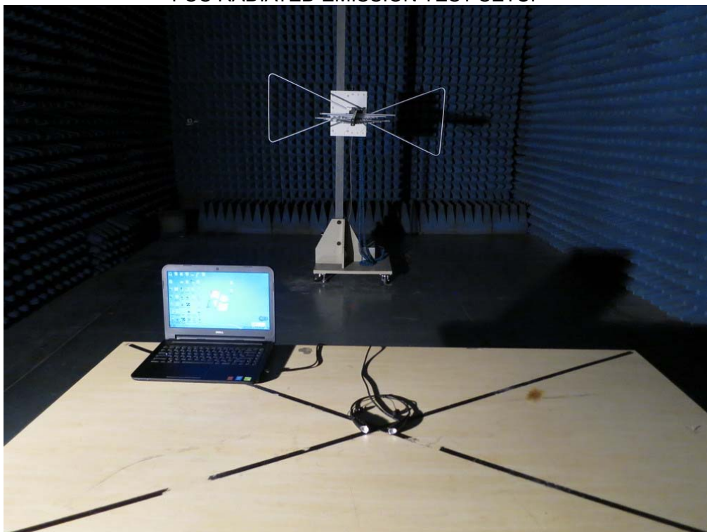
FCC RADIATED EMISSION TEST SETUP
