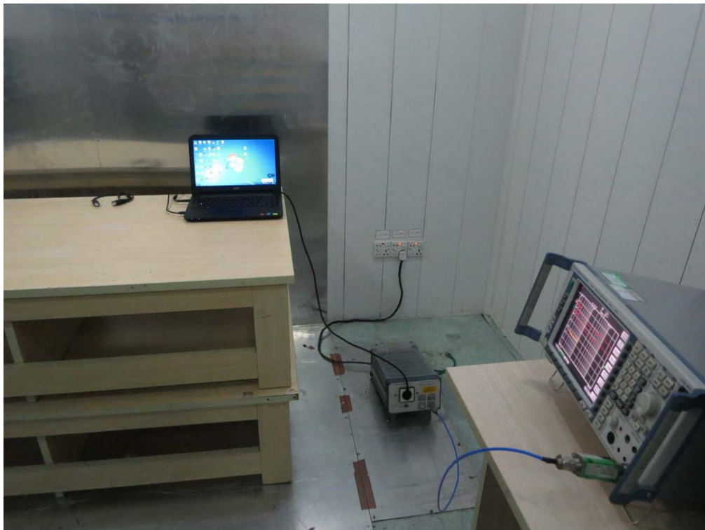
FCC RADIATED EMISSION TEST SETUP
