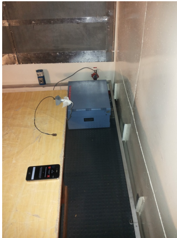
Photograph 8.1.2 Setup for conducted emission measurements
