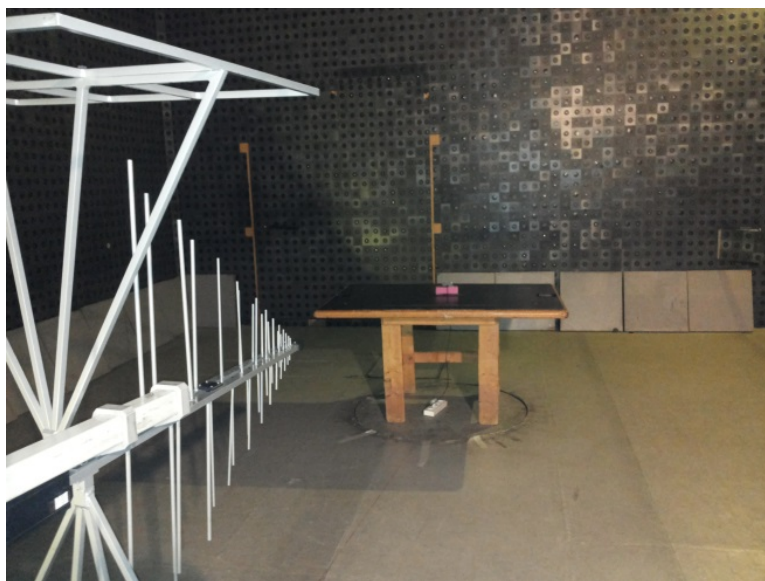
Photograph 8.2.2 Setup for radiated emission measurements
