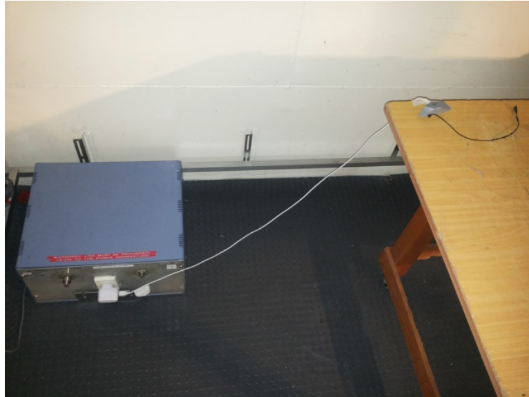
Photograph 8.1.2 Setup for conducted emission measurements
