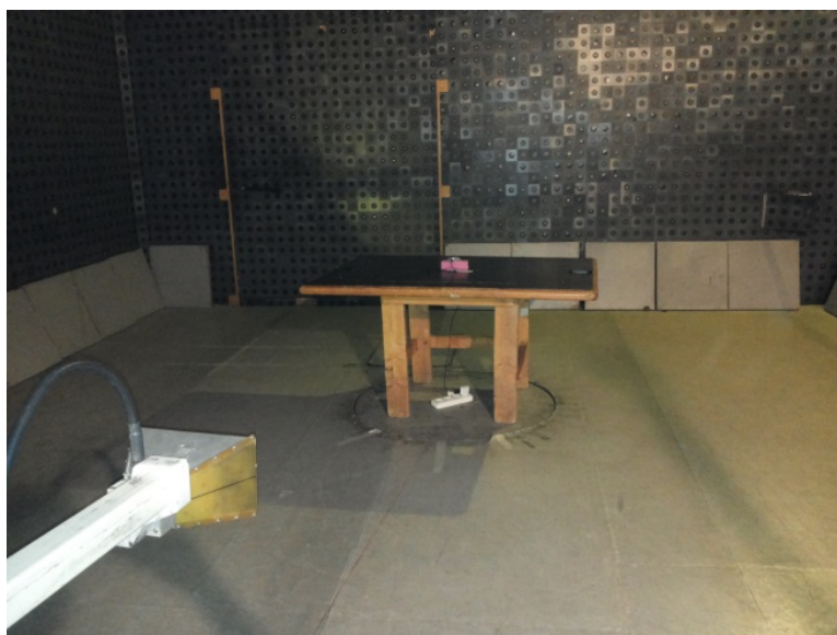
Photograph 8.2.2 Setup for radiated emission measurements
