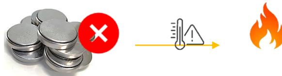
The entire surface of lithium button batteries is conductive, and they can short-circuit and **catch fire quickly**. NEVER store these batteries together without protection.
