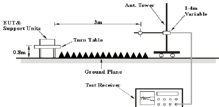
The radiated emission tests were performed in the 3 meters chamber test site A for the range 30MHz to 1GHz and the 3 meters chamber test site A for above 1GHz, using the setup accordance with the ANSI C63.4-2014. The specification used was the FCC Part 15.109 Class B limits.
