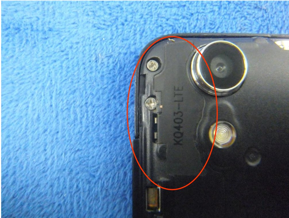
LTE - Antenna View
