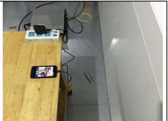
Conducted Emissions Test Setup Side View
