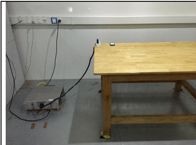
Conducted Emissions Test Setup Front View
