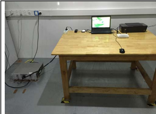
Conducted Emissions Test Setup – Front View
