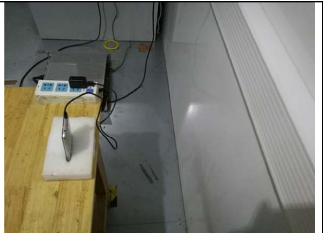
Conducted Emissions Test Setup Side View
