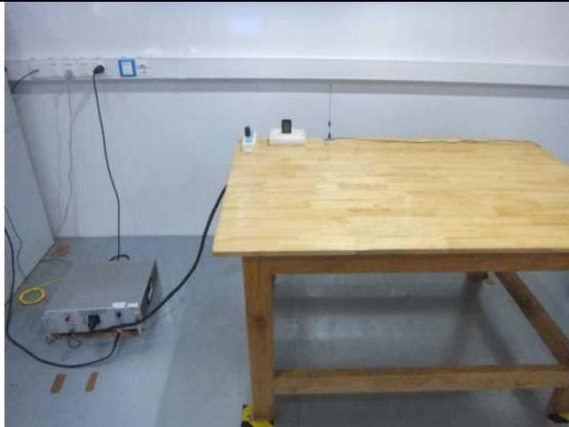
Conducted Emissions Test Setup Front View
