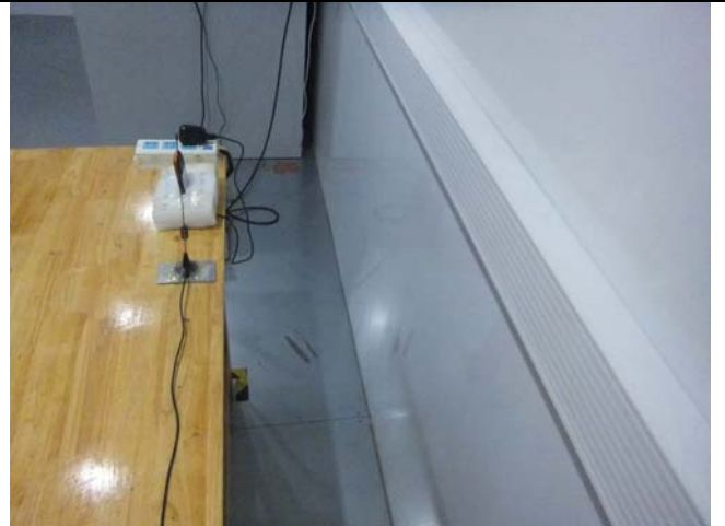
Conducted Emissions Test Setup Side View
