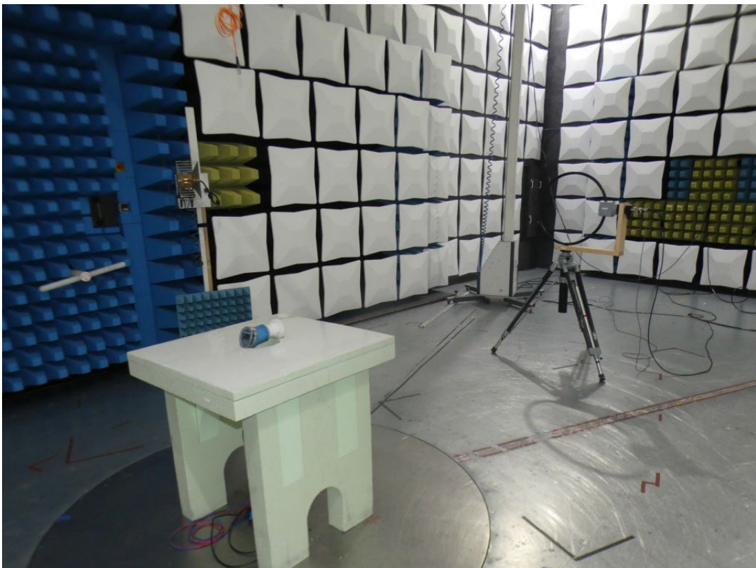
Photo 2: Test setup for radiated measurements below 30 MHz
