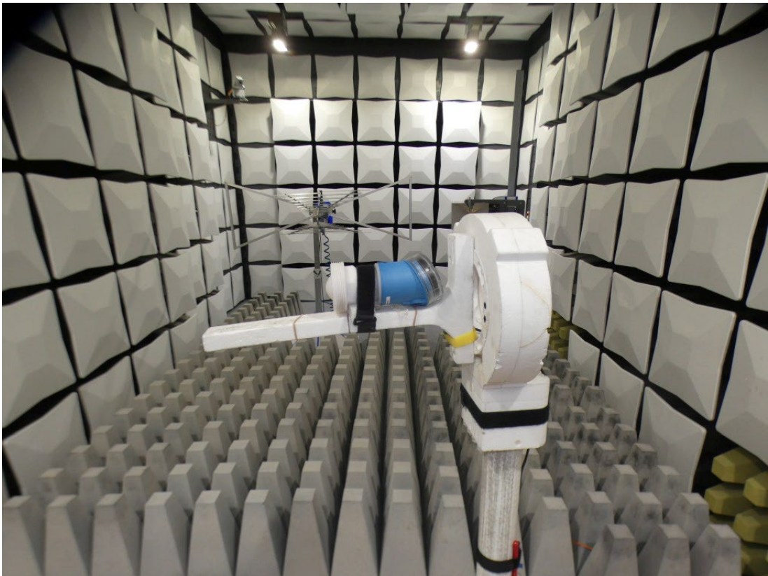
Photo 5: Test setup for radiated measurements above 18 GHz
