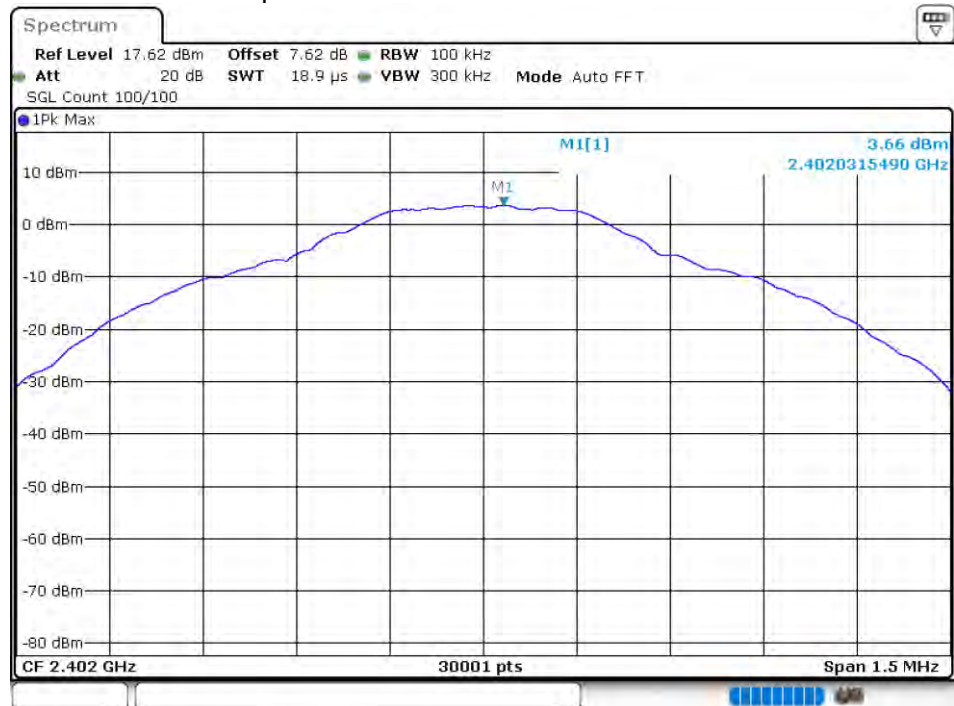
Tx. Spurious NVNT 1-DH5 2402MHz Ant1 Ref
